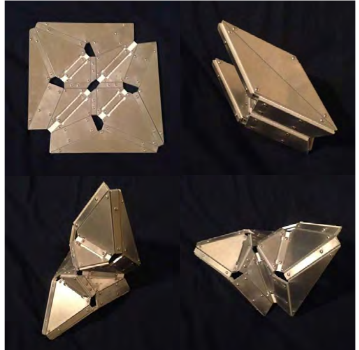
FIGURE 13. Axially varying volume trimming applied in combination with the offset crease method to produce a thick folding bird base from aluminum.
