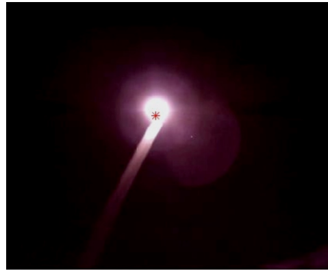
Fig. 5. A camera frame showing a detected lamp centroid at the red star. This image processor is just one of many that can be used to identify city assets.
