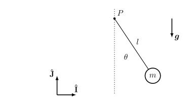
Consider a pendulum consisting of a point mass m and rigid rod of length L with negligible mass moving in the presence of gravity. The pivot point P of the pendulum is not fixed but follows some non-zero trajectory  ${}^{O}\boldsymbol{r}_{P}(t)$ . Derive the equations of motion for the system. Then derive the equations of motion for the specific pivot trajectory  ${}^{O}\boldsymbol{r}_{P}(t) = A\cos(\omega t)\hat{\mathbf{J}}$ .
