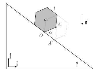
A pencil with regular hexagonal cross-section, mass m, and side length l is placed on a no-slip inclined surface. Define I as the moment of inertia of the pencil about an edge. Given that  $\theta > 30^{\circ}$ , it begins to rotate due to gravity.
