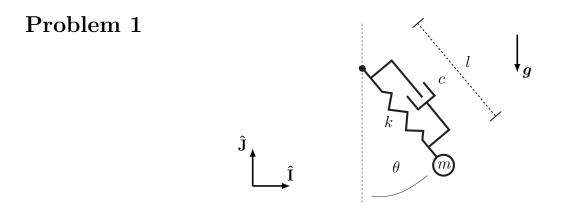
A small ball of mass m hangs from an elastic string which can be modeled as a spring with coefficient k in parallel with a dashpot with coefficient c. The spring has a natural length l. Consider the motion of this pendulum in a plane in the presence of gravity. Derive the equations of motion for the system. Are the equations of motion coupled in general? Are the equations of motion coupled for small angles?
