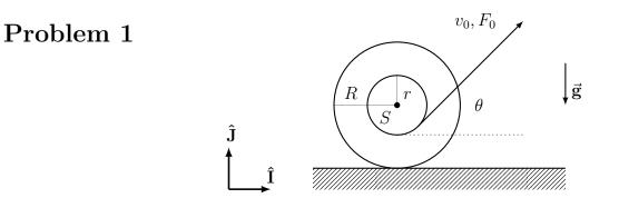
A spool of mass m and moment of inertia about its center I, with inner radius r and outer radius R sits on a table, initially at rest but can roll without slipping. A thread wrapped around the inner radius is pulled at an angle  $\theta$  from the horizontal. Find the velocity of the center of the spool S with respect to the ground as a function of both time and angle under the following conditions:
