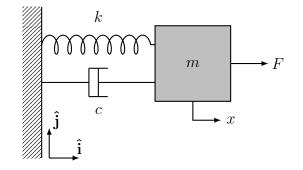
Mass *m* is connected to a fixed wall by a spring *k* and dashpot *c* in the absence of gravity. Initially the system is at rest with x(0) = 0 and  $\dot{x}(0) = 0$ . At time t = 0, a constant force  $F\hat{i}$  is exerted on the mass.
