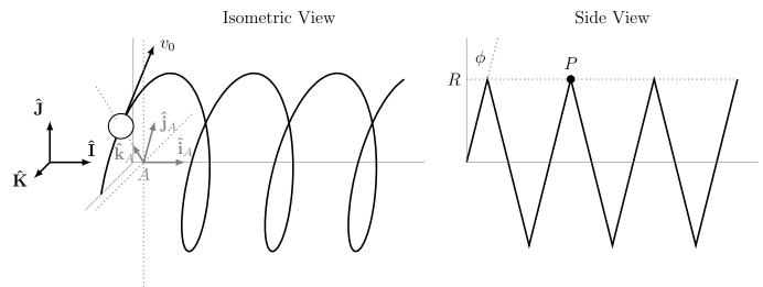
A roller coster car travels with constant tangential velocity  $v_0$ , on a helical track with radius R and pitch angle  $\phi$ . What is the velocity and acceleration of the car with respect to the ground when it reaches point P, the second peak of the helical track?
