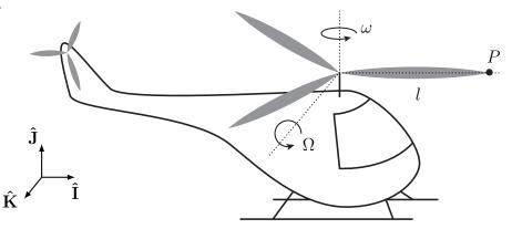
A helicopter is hovering in the air. The blades of its main rotor have length l and are spinning with angular velocity  $\omega$  with respect to the helicopter. At the time shown, the helicopter is also tilting upward with constant angular velocity  $\Omega$  with respect to ground. Find the velocity and acceleration of point P at this instant.
