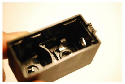
See that locking tab that held the potentiometer in place? It's going to get in the way, so remove it!
