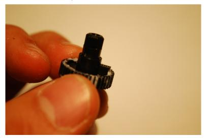
The output gear has a tab that limits its rotation to 180 degrees. This needs to be removed.
