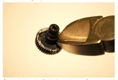
Clip the limiting tab off with diagonal cutters. Remove as much as possible or the gears may scrape inside the motor.
